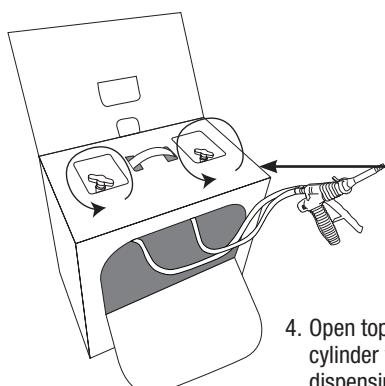
4. Open top flap of box to expose cylinder valves. Extend attached dispensing unit hose assembly.
