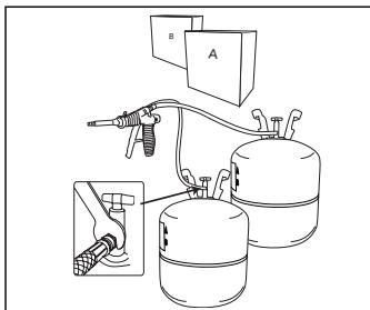
2. Thread red coded hose to A-component tank and black coded hose to B-component tank and tighten with supplied 9/16" wrench.
