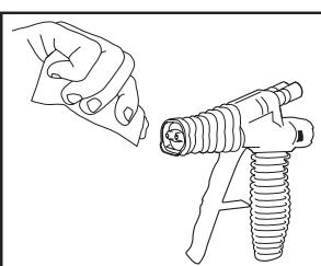
1. Before attaching nozzle, use petroleum jelly on face of gun. After attaching nozzle, spray into "test shot" receptacle.
