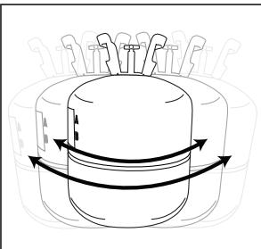
1. Shake kit for 1–2 minutes before use to ensure proper mixing, see TDS for formula specific shaking and temperature recommendations. Chemical should be between 75–85°F (24–29°C).
