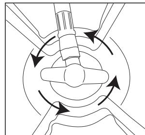
3. Open the valves completely by turning the valves COUNTER CLOCKWISE. Tank valves must be upright during use.
