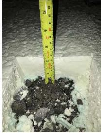
Heatlok Soya HFO is 100% in contact with its substrate making it very solid to walk on. Different thickness can be applied depending on the required R-value. 2" as demonstrated above is a common application.
