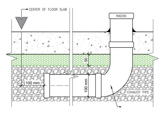
PERFORATED PIPE IN THE GRAVEL UNDER THE SLAB RESIDENTIAL APPLICATION
