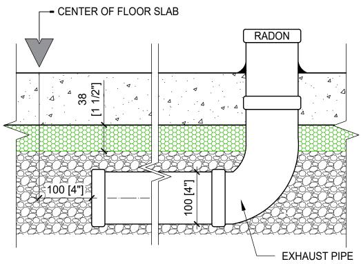
PERFORATED PIPE IN THE GRAVEL UNDER THE SLAB RESIDENTIAL APPLICATION
