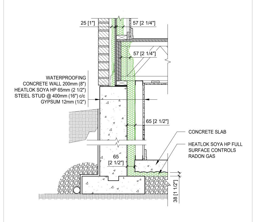
$38 \text{mm} (1 \ 1/2") \text{ UNDER SLAB - INTERIOR FOUNDATION APPLICATION}$  RESIDENTIAL APPLICATION
