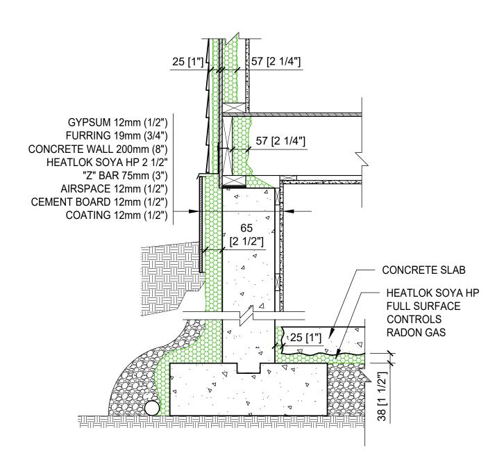
$38 \text{mm} (1 \ 1/2") \text{ UNDER SLAB - EXTERIOR FOUNDATION APPLICATION}$  RESIDENTIAL APPLICATION
