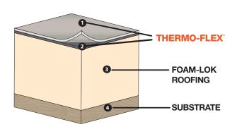
Choosing to spray foam your roof can reduce the wear and tear that occurs with traditional roofing materials. Applying Huntsman Building Solutions Thermo-Flex™ acrylic roof coating system preserves the life of commercial and residential roofs. This advanced insulation is applied to any design and most substrates, sealing the building envelope to stop heat transfer through the roof deck.
