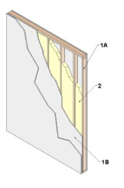
WOOD STUDS: Install nominal 2-inch-by-4-inch Number 2 Southern Yellow Pine wood studs spaced maximum 16 inches on center.
