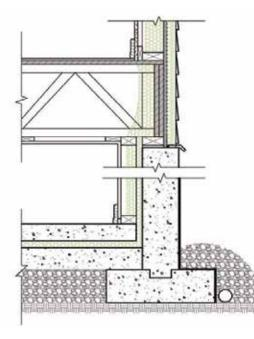
Detail for sealing a bearing wall or an existing divider.
