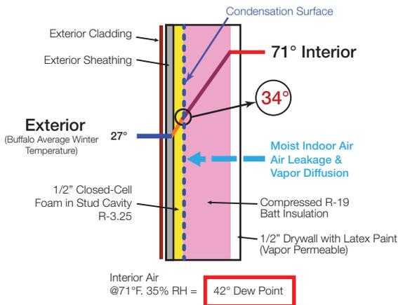
This wall section poses the risk of condensation forming in the wall, even at average winter temperatures. In addition, the closed-cell spray foam is not at an acceptable thickness to achieve a Class II vapor retarder rating. This system will require an additional vapor retarder on the interior side of the fiberglass insulation to lower the risk of moisture problems.
