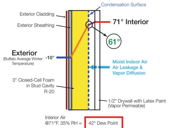
This wall section is properly designed using closed-cell spray foam. The applied thickness meets the minimum required R-value and is adequate to achieve a Class II vapor retarder rating. This wall section effectively places the vapor retarder layer on the interior side of the wall, and removes most risk for condensation forming.
