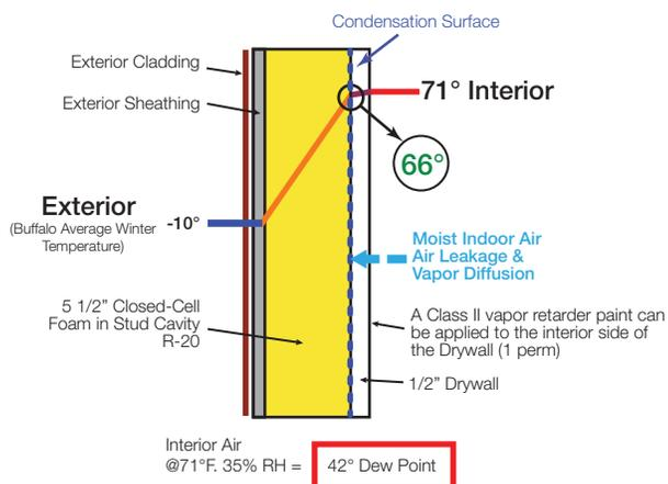
This wall section is properly designed using open-cell spray foam insulation and a Class II vapor retarder (required in Climate Zones 5, 6, 7, 8 and Marine 4), applied to the interior side of the wall assembly. This wall assembly meets all prescriptive building code requirements for R-value and vapor retardance, and removes most risk for condensation forming.
