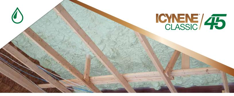
Icynene® Classic 45 is a High Yield OC spray applied foam when installed following application guidelines, adheres tenaciously to framing members and substrates. Icynene Classic 45 is a low density, open celled, flexible, 100% water-blown polyurethane foam insulation. It is capable of being installed in unvented attics without an ignition barrier or coating.
